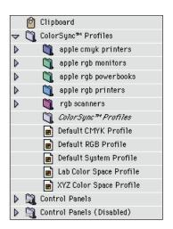
ColorSync software consists of profiles, a control panel, a monitor calibration assistant, and extensions allowing color preparation and preview at the desktop.
